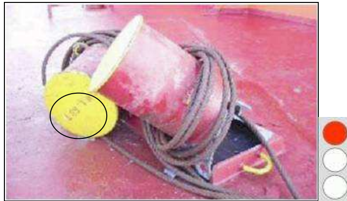
This was a 65t SWL bollard!
