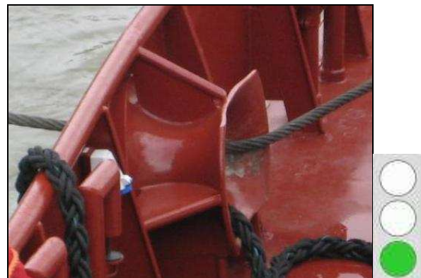
Chock reinforced by stiffeners
